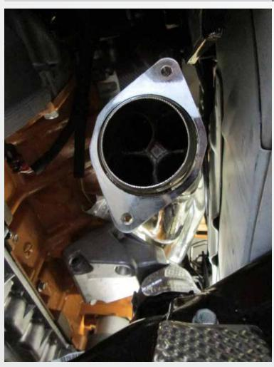
Install BBK headers with supplied gaskets and hardware making to use dipstick bolt and nut. Re-attach alternator brace and install motor mount. Then install factory head pipes. Install factory plastic shields and start vehicle checking for any leaks. Recommended to re-torque all header fasteners the following day after a couple heat cycles.
