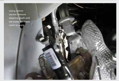
Place vehicle on flat surface making sure to use jack stands when working on vehicle. We recommend spraying all Fasteners with WD40 or similar to make fastener removal easier.
