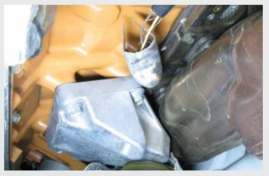
Repeat same steps as driver's side but you will also have to remove dip-stick and remove alternator brace bracket. (Note: you will be re-using dipstick bolt and nut for install).
