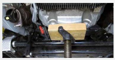
Safely support engine for removal and install of motor mounts.
