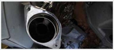
Install BBK headers using supplied hardware and gasket with 12mm socket/wrench. Re-install motor mount and steering shaft.
